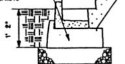
ALTERNATE FOOTING DETAIL FOR 6' 0" HERC. STD. WALL
